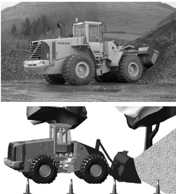
Fig. 1: Loading procedure; reality and simulation, the upper illustration is from Volvo Construction Equipment, Sweden
