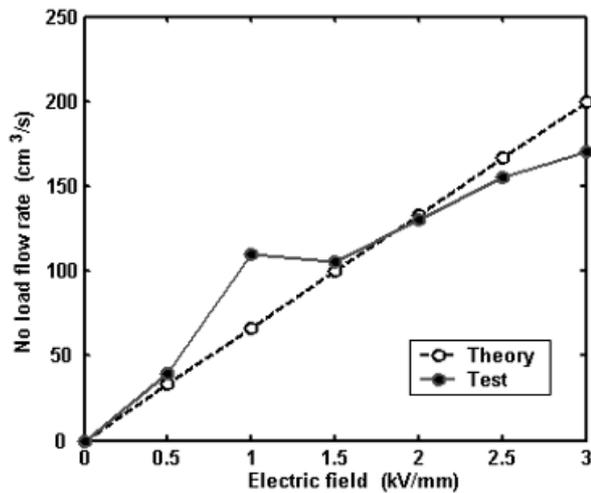
Fig. 5: The relationship between no load flow rate and electric field strength
