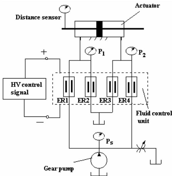
Fig. 4: Configuration of experimental apparatus
