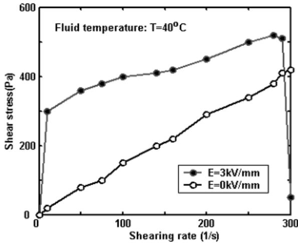
Fig. 3: Characteristic of ER fluid
