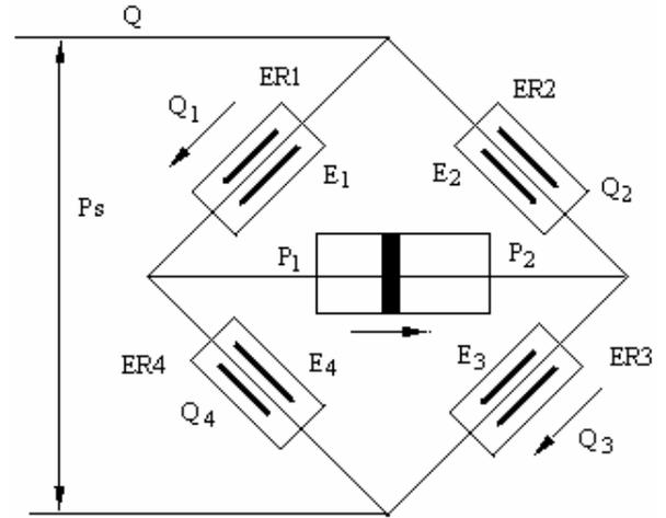
Fig. 2: ER fluid control unit
