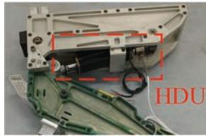
**Figure 7** Hydraulic drive unit.
