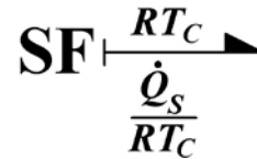
Fig. 7: Bond-graph model of heat transfer through wall
