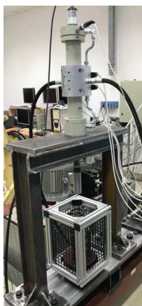
Figure 2 Test rig with the integrated hydraulic actuator for spring stiffness measurement.
