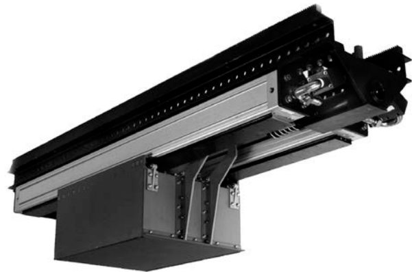
Fig. 2: Pneumatic slide acceleration mechanism with the two double acting pneumatic linear drives, the plain bearing guides, the slide box and the pneumatic cylinder driven flap opening mechanism
