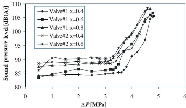
Fig. 12: Sound pressure level of noise in converging flow
