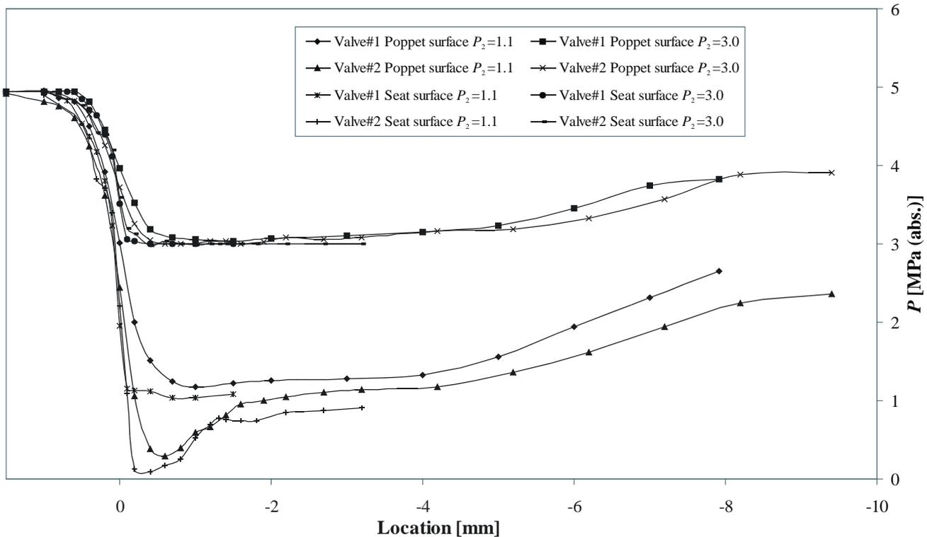
Fig. 11: Pressure distribution in converging flow
