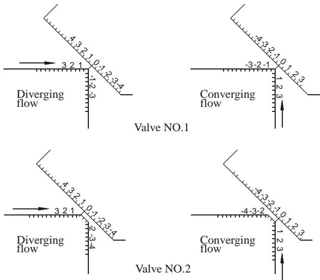
Fig. 10: Systems of coordinates in pressure distribution measurements
