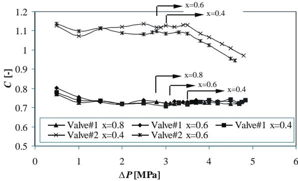
Fig. 9: Discharge coefficients in converging flow
