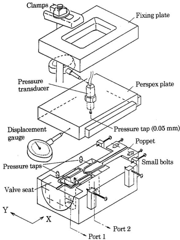
Fig. 1: Structure of half cut test model
