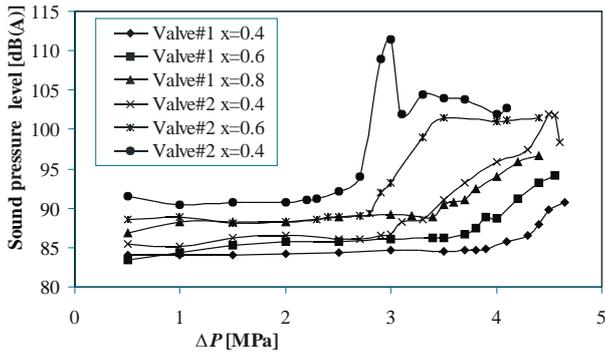
Fig. 8: Sound pressure level of noise in diverging flow
