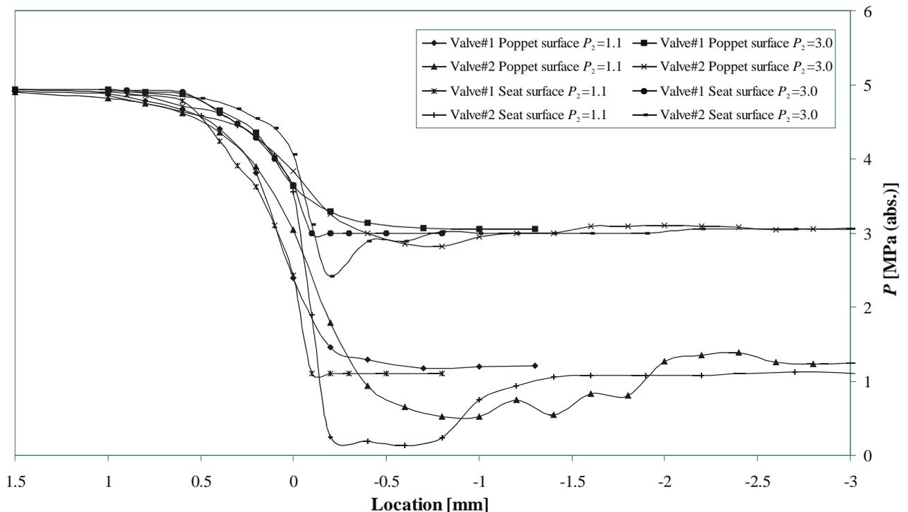
Fig. 7: Pressure distribution in diverging flow
