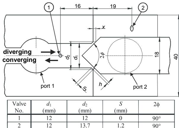
Fig. 2: Overview of main part and the important dimensions
