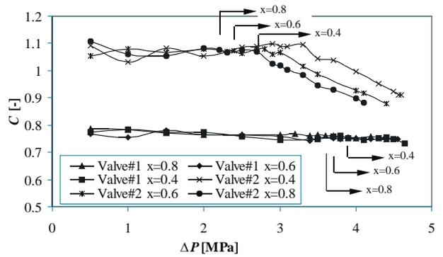
Fig. 6: Discharge coefficient in diverging flow
