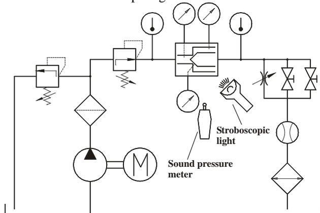
Fig. 3: Hydraulic circuit used for tests
