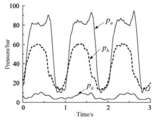
Figure 3 Pressure curve of pump and valve coordinated control system.
