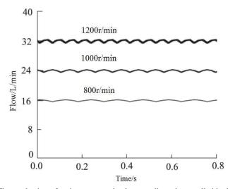
**Figure 4** Flow pulsation of series pump and valve coordinated controlled hydraulic system under 25 Bar.
