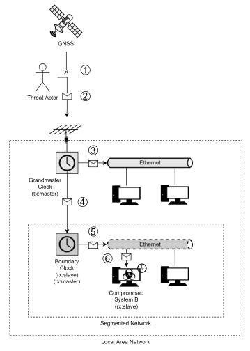
Figure 6 Threat Scenario leveraging the Precision Time Protocol as carrier for data infiltrating covert channels.
