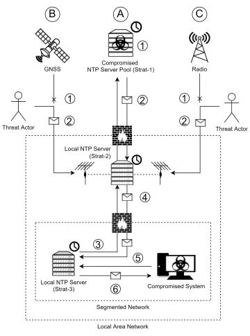
Figure 5 Threat Scenario leveraging the Network Time Protocol as carrier for data infiltrating covert channels.
