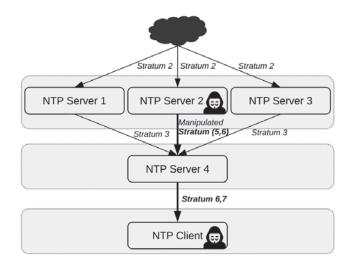
**Figure 4** The covert channel two uses the stratum values in NTP server packets to send hidden information from a malicious NTP server (2) through an non-involved server (4) to a client. Server 4 is requesting time from three upstream servers (1,2,3), but only server 2 is malicious.
