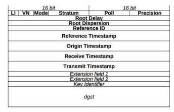
Figure 1 The structure of an NTP packet. 13 fields are mandatory, the two extension fields and the MAC field (key identifier plus dgst) are optional.
