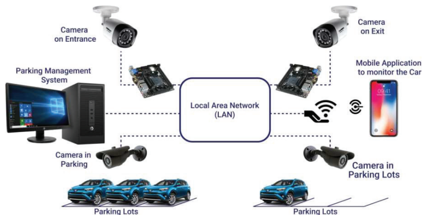
Figure 1 Structure of smart parking system.
