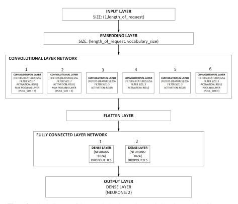
Figure 2 Block diagram of the convolutional neural network detection model architecture.
