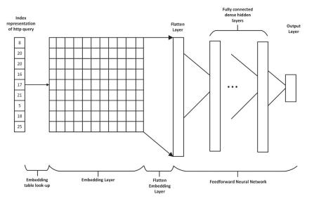
Figure 1 Deep neural network detection model architecture showing the embedding layer and feed forward neural network.
