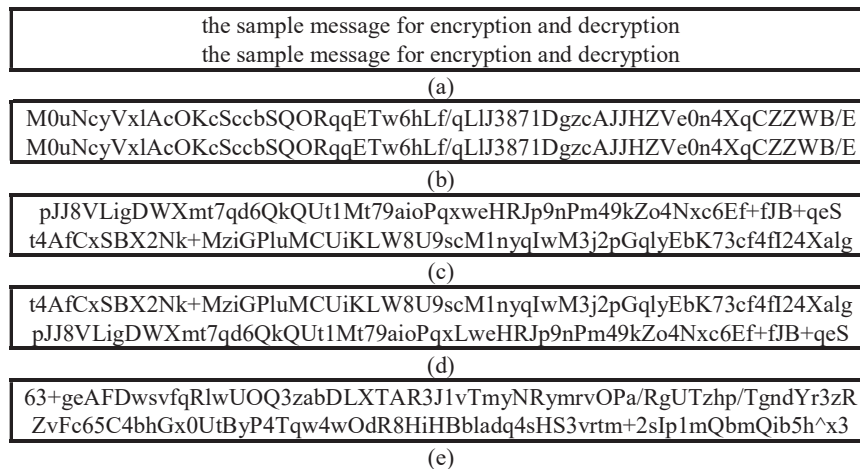
Figure 4 (a) A message considered for encryption using original TEA. (b) The encrypted message using TEA. (c) The same message encrypted using ATEA. (d) The decrypted message after changing one number in initial sequence. (e) The decrypted message after changing one irreducible primitive trinomial.
