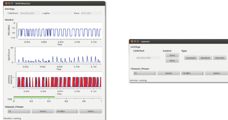
Figure 10 Graphical user interface of remote interface from sensor node (left) and jammer (right) application
