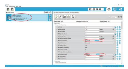
Figure 4(a) (1) Zigbee module configured as coordinator.
