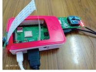
(b) Raspberry PI communicating with Zigbee configured as coordinator
