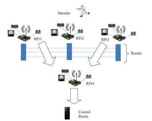
**Figure 1** Autonomous Border Surveillance System with Raspberry PI wireless sensor nodes equipped with PIR, Ultrasonic and PI camera sensors for identifying the Intruders.
