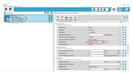
Figure 4(b) (2) Zigbee module configured as router.
