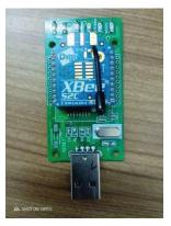
Figure 3 Zigbee module (XBee S2C).
