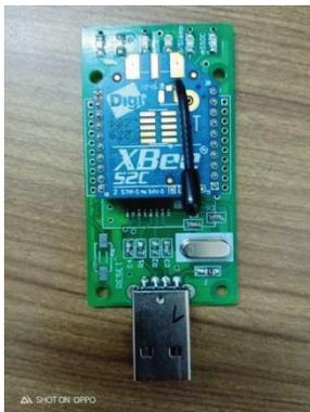
**Figure 3** Zigbee module (XBee S2C).
