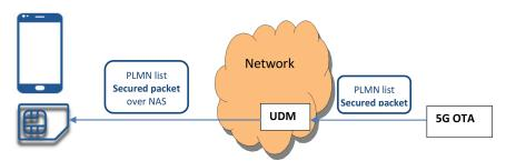
Figure 3 Steering of roaming with the USIM.
