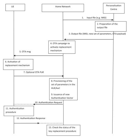
Figure 4 Key replacement procedure.
