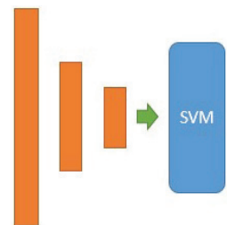
Figure 4 Three stacked LSTM with SVM in the last layer.
