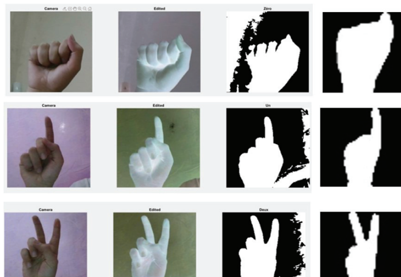
Figure 10 Color image converted to binary via a grayscale image, binary image with noise and filtered binary image.
