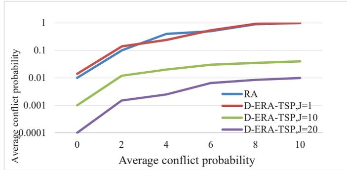
**Figure 9** Relationship between average collision probability and number of terminal devices ( $M = 60$ ).
