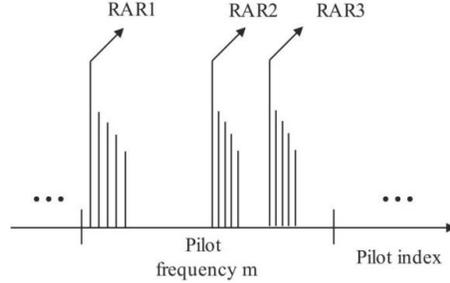
**Figure 3** Schematic diagram of processing multiple peaks of the same pilot.
