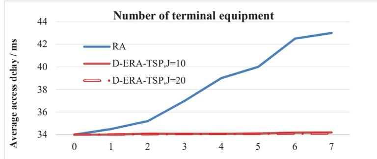
**Figure 11** Relationship between average access delay and number of terminal devices (number of antenna units  $M = 60$ ).
