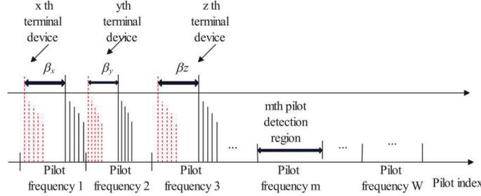
**Figure 2** Schematic diagram of pilot detection of ERA-TSP scheme.
