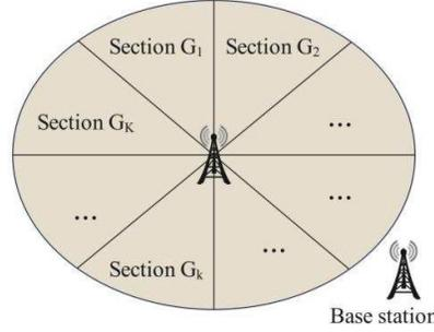
**Figure 1** Schematic diagram of sector division in a cell.
