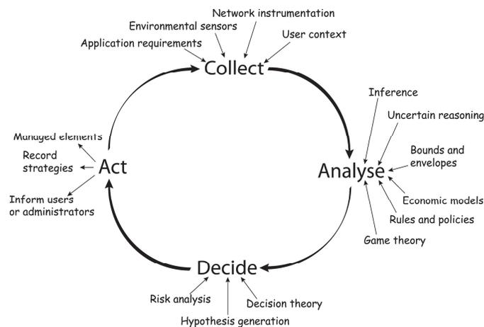
**Figure 1** Autonomic control loop [23].
