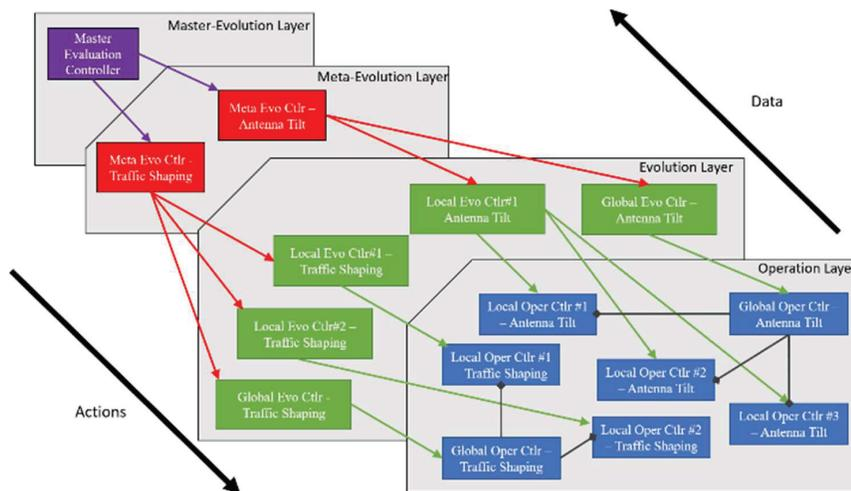
Figure 4 Example controller hierarchy split by layer.
