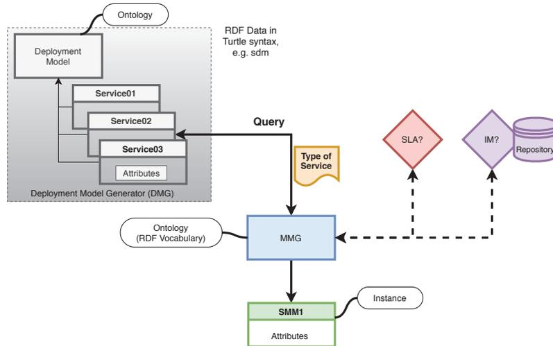
**Figure 2** System Architecture.
