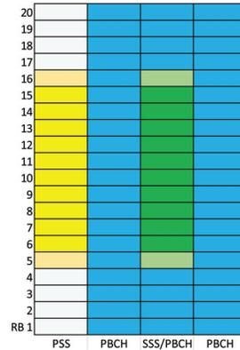
**Figure 5** Illustration of SS block.
