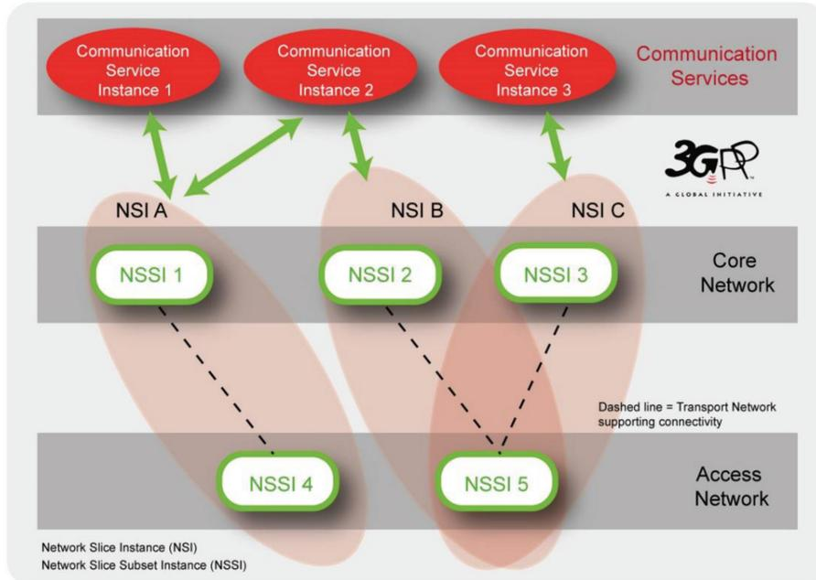
**Figure 1** Communication service instances provided by multiple NSIs.
