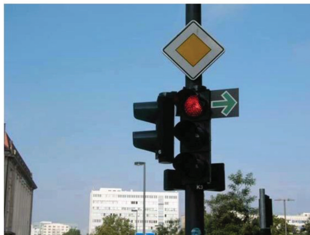
Figure 7 Traffic signs attached to traffic signal (Germany)
