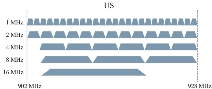
Figure 2 IEEE 802.11ah channelization for the US.
