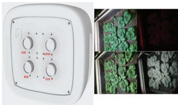
Figure 4 MSI-RPi setup (L-R: The camera setup front-view, Acquired images – 1st image (550 nm), 2nd image (1070 nm), 3rd image (RGB), 4th image (725 nm)).
