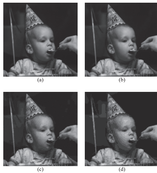
Figure 12 JPEG Compression Results for Child Image (a) Original image (b) Decompressed image with Quality Factor = 1 (c) Decompressed image with Quality Factor = 5 (d) Decompressed image with Quality Factor = 10.
