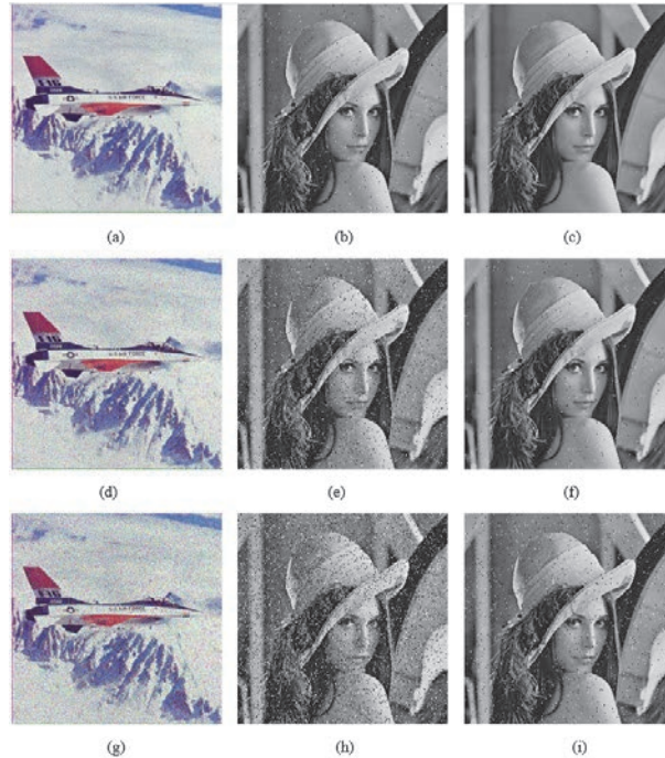
Figure 12 Salt and Peppers noises d = 0.01 : (a) stego image (b) extracted secret image without recovery (c) extracted secret image after recovery Salt and Peppers noises d = 0.05 : (d) stego image (e) extracted secret image without recovery (f) extracted secret image after recovery Salt and Peppers noises d = 0.1 : (g) stego image (h) extracted secret image without recovery (i) extracted secret image after recovery.
