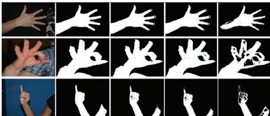
Figure 6 Visual comparisons using different skin segmentation methods on HGR dataset. (From Left to right): Original image, ground truth, DeepLabV3+ [12], Proposed detector, static rule-based method [13].
