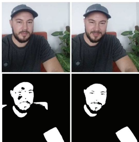
Figure 7 Motion based Adaptive Thresholding. (Left): frame at time t_0 , (Right): Frame at time t_0+5s .
