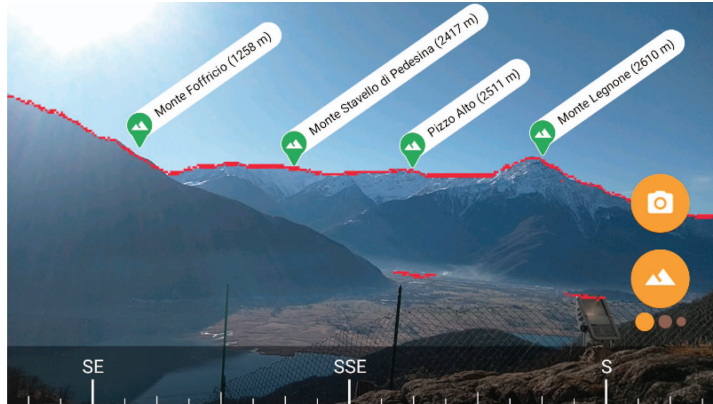
Figure 5 The skyline extracted from the computer vision module from the frame of Figure 2.
