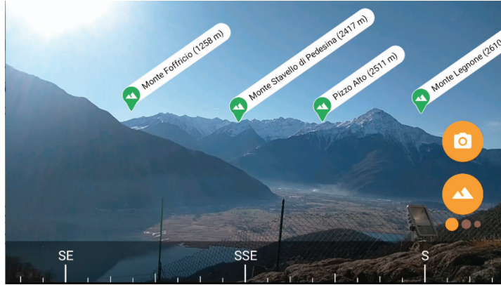
Figure 3 A soft error that cause peak labels to be misplaced.
