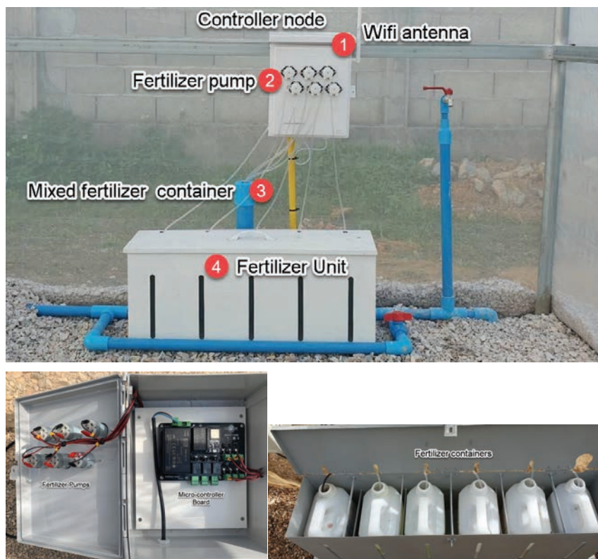
Figure 6 Installation of the system at the melon plant.
