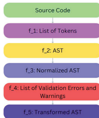
Figure 1 Using a parser library, turn a smart contract into an AST. These libraries will convert the code to a tree structure, which can subsequently be manipulated or analysed.
