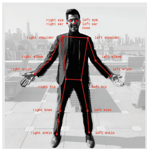
Figure 1 Main joints of the human body (key points) that are detected by PoseNet . Available at [9].
