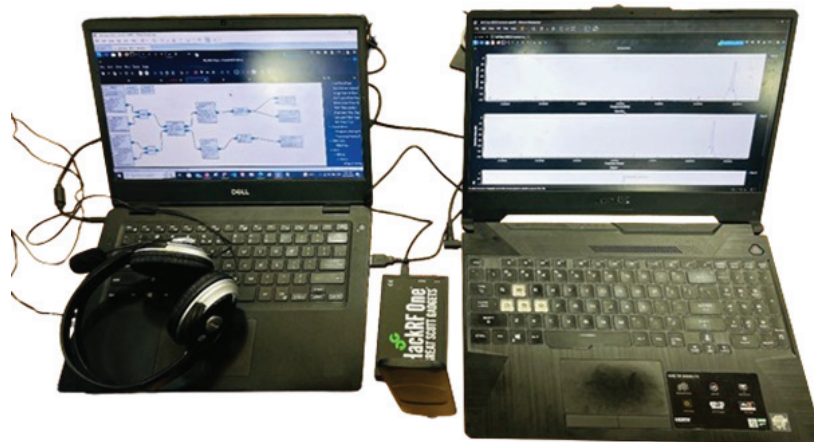
Figure 5 Hardware implementation using HackRF SDR.
