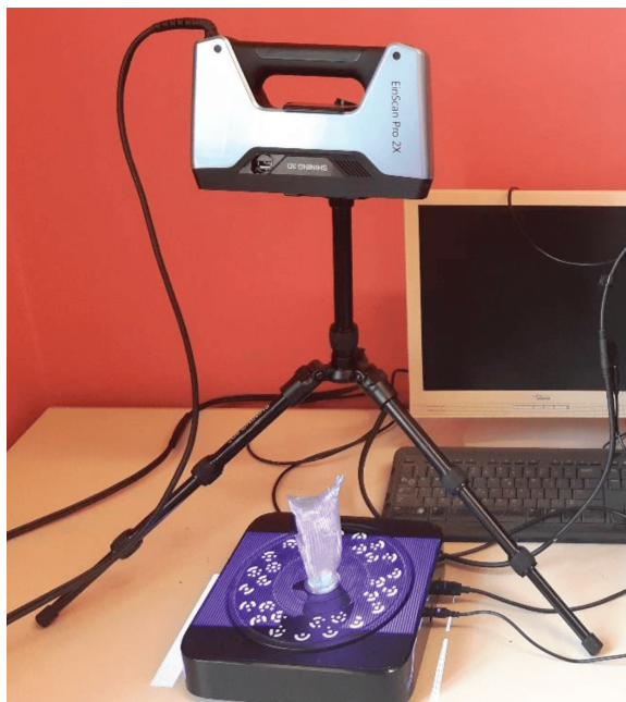
Figure 10 The scanning of a glass artifact utilizing a portable 3D scanner [40].
