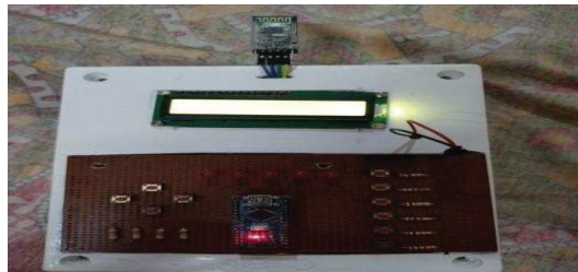
Figure 1 Rover controller with liquid crystal display, LEDs, push button.
