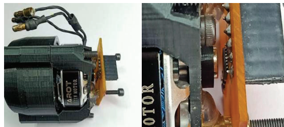
Figure 4(b) AS5147 breakout board mounting the actuator back plate, close up view of encoder above diametric magnet.
