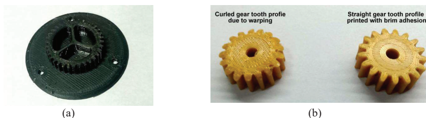
Figure 8 (a) & (b): Second stage sun gear merged with first stage planet carrier allows to have reduced no. of joining links ; Bottom View before and after build plate adhesion.
