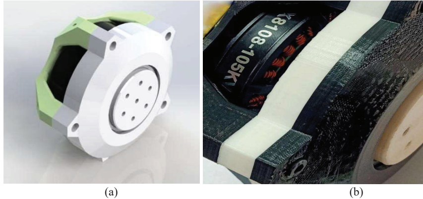
Figure 6 (a) & (b): Actuator Iteration Design; ex8108-105KV B.L.D.C. as base motor.
