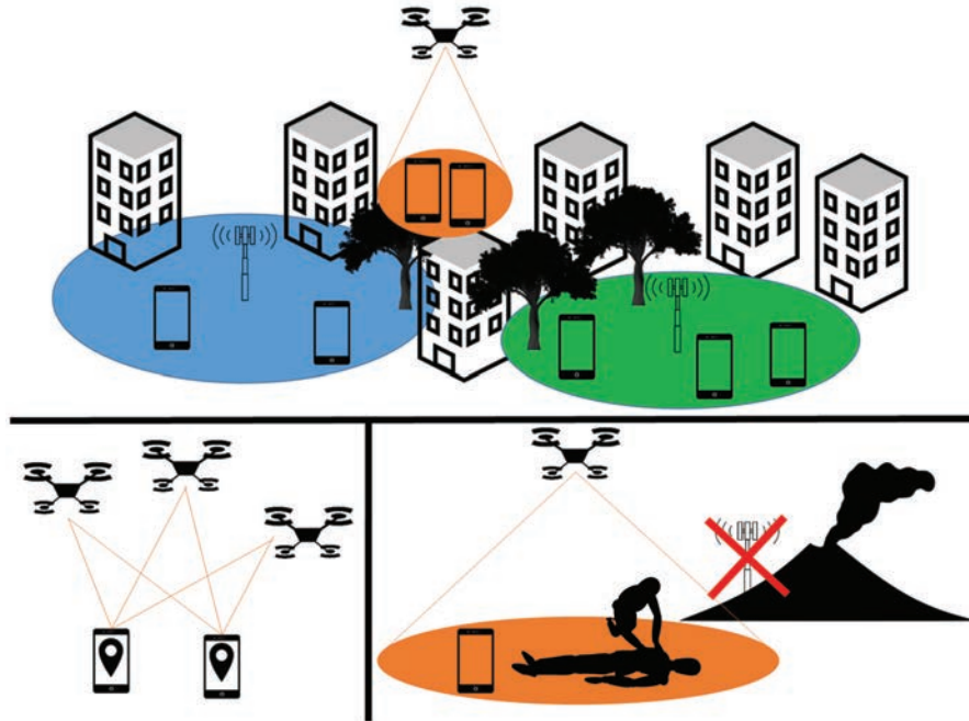
Figure 4 Aerial Base Station use cases. Top: Future communication networks; Bottom, Left: Localization service; Bottom, Right: disaster scenario.
