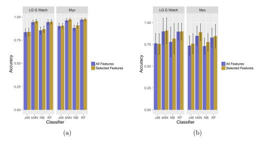
Fig. 5. The recognition accuracies for the first gesture variant for both devices, each classifier and all features as well as for the selected features. The evaluation was done with (a) 10-fold cross-validation with 10 repetitions and (b) with leave-subject-out cross-validation.
