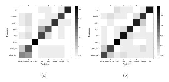
Fig. 9. The confusion matrices for the second variant of the recorded gestures with leave-subject-out cross-validation for the best classifier of (a) the Myo armband and (b) the LG G Watch (the Random Forest for both) with only the selected features.
