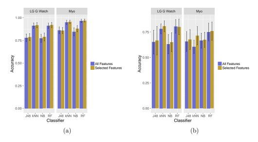
Fig. 6. The recognition accuracies for the second gesture variant for both devices, each classifier and all features as well as for the selected features. The evaluation was done with (a) 10-fold cross-validation with 10 repetitions and (b) with leave-one-subject-out cross-validation.
