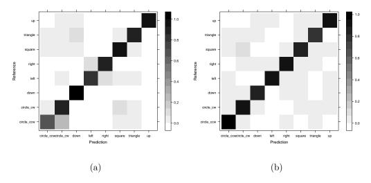
Fig. 8. The confusion matrices for the first variant of the recorded gestures with leave-subject-out cross-validation for the best classifier of (a) the Myo armband (kNN with k=9) and (b) the LG G Watch (kNN with k=7) with only the selected features.
