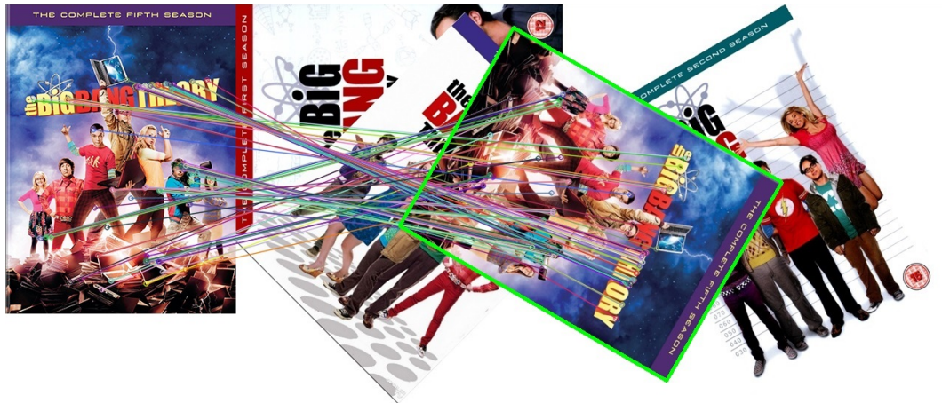
Fig. 1. Example of matching a pattern in an image (left) on a set of images where the pattern is inserted (right).
