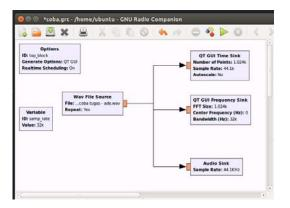
Figure 1. GRC block on GNU Radio for sampling rate adjustment for audio processing.
