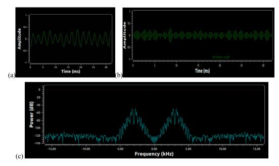
Figure 6 (a) Input audio (piano instrument), (b) AM modulated signal, and (c) Frequency spectrum of modulated signal.
