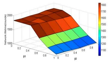
Figure 5 Plot of network lifetime with 100% sensing coverage versus  $\beta$ 1 and  $\beta$ 2 when w1=0.8 and w2=0.2.
