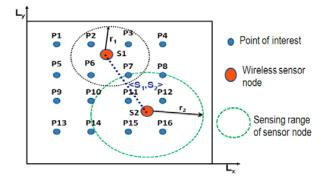
Figure 2 Example for the coverage model of sensor nodes.
