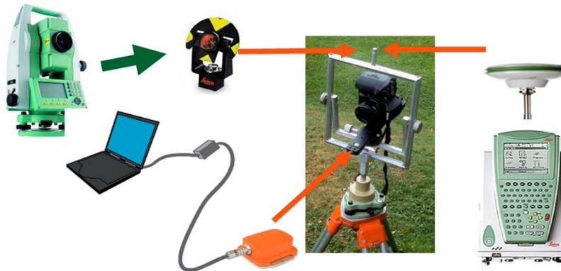
Figure 3 The calibrated head used for georeferenced panorama acquisition.
