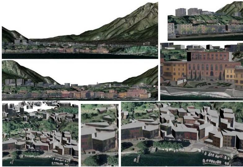
Figure 8 3D texture mapping of DTM and spatial database (building layer) from multiple GeoPans.
