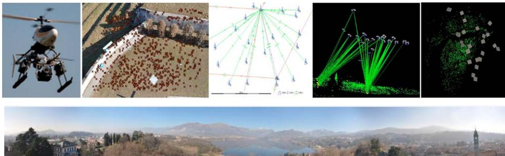
Figure 5 Some phases of the creation of the georeferenced UAV panorama (top) and the final GeoPan (bottom).
