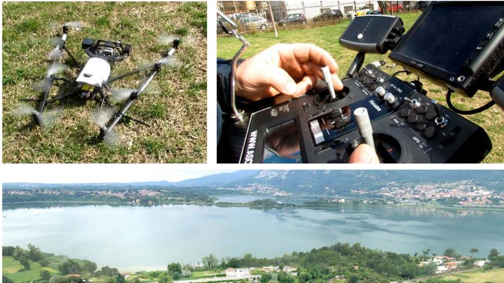
Figure 6 The Falcon 8 and the ground station (top). The GeoPan from image stitching (bottom).
