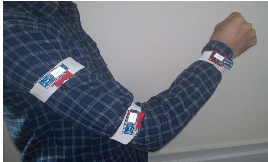
Figure.2. Placement of sensors on the test subject's arm
