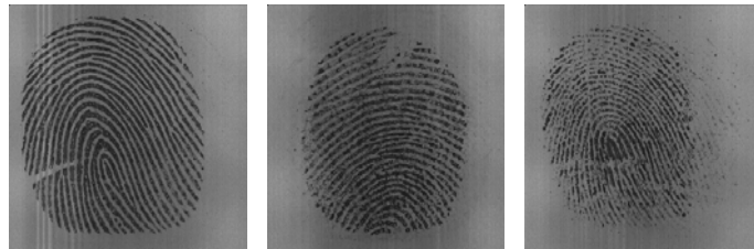
Figure 4. Two typical fingerprints of different quality. On the left a fingerprint image of good quality ( GI=82.01 ), on the center a fingerprint image of medium quality ( GI=55.01 ), while on the right a fingerprint image of bad quality ( GI=0 ).
