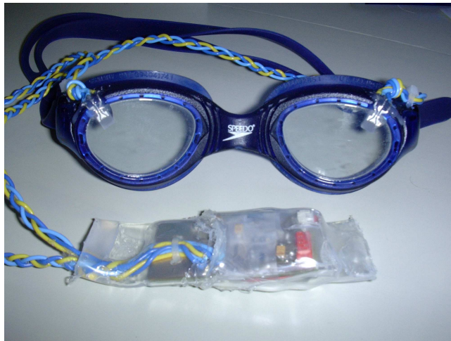
Fig. 1. Goggles with one bi-color LED[2]
