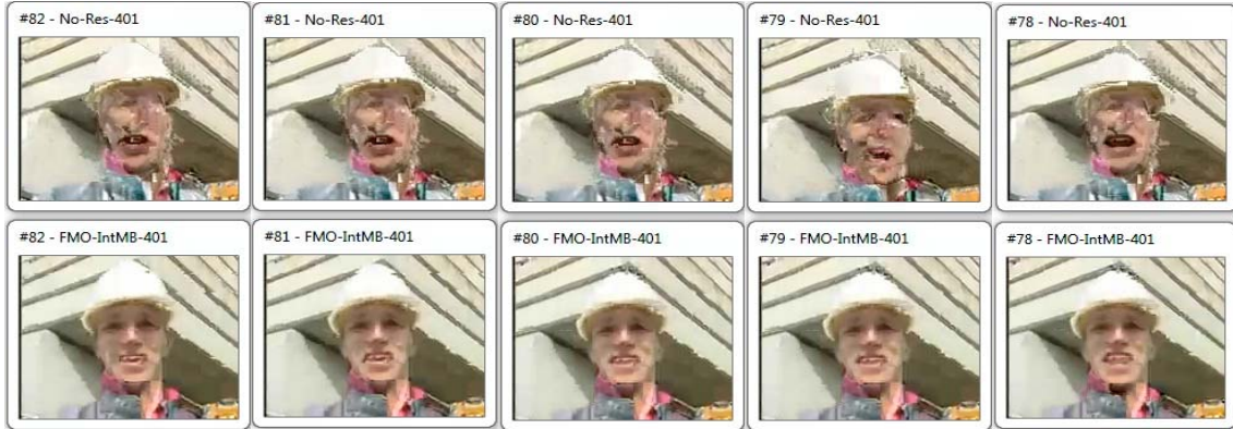
Figure 4 Visual comparison of No-res and FMO-IntMB for selected frames of the “Foreman” sequence.
