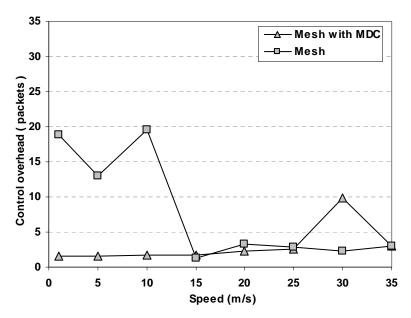
Figure 10 Control overhead with variation in speed.
