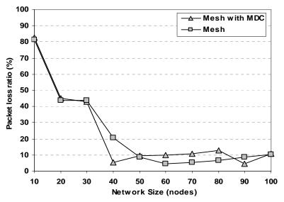
Figure 5 Packet loss ratio, varying node numbers.
