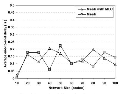
Figure 6 Average end-to-end delay, varying node numbers.
