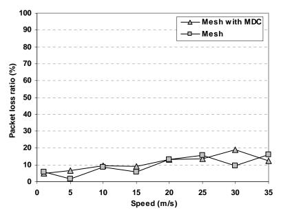
Figure 8 Packet loss ratio with variation in speed.
