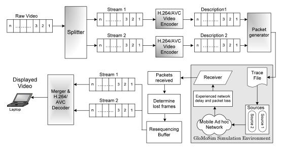
Figure 4 H.624 and GloMoSim Simulation Environment for MDC, after [10]
