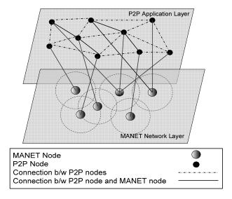
Figure 1 An example of a P2P application overlay over MANET, after [8].
