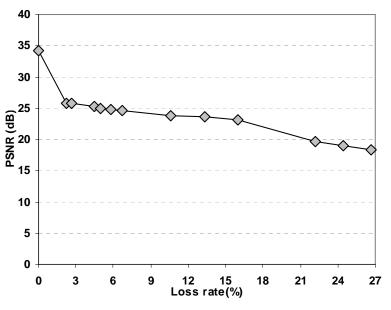
Figure 11 Video quality for MDC by packet loss ratio.
