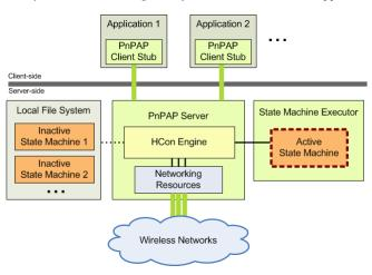
Figure 2 Structure of HCon.
