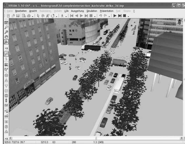
Fig. 5. VISSIM graphical user interface and a 3D traffic model
